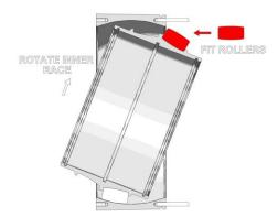
Rotate the inner race and the first track of roller in opposite direction so the other roller track is just exposed at the upper edge and a roller can be placed in the track.
