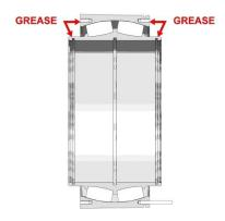
Fit each V-seal and seal carrier.
