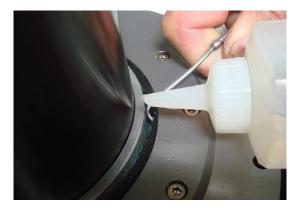
Add a few drops of the silicone oil supplied through the gap in the seal. Rotate the rudder back and forth to help distribute the oil through the bearing. The oil
